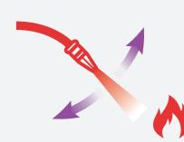
weep the nozzle or hose from side to side until the fire is out, starting at the recommended distance. Move forward or around the fire area as the fire diminishes. Watch the area in case of re-ignition.
