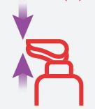
**SQUEEZE** the operating lever to discharge the fire extinguishing agent.
